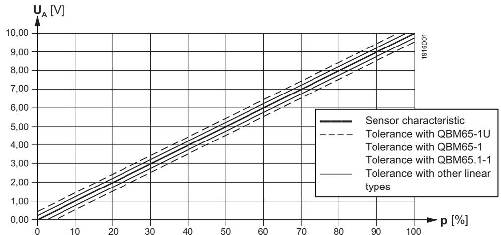
Extracting-the-root output and total tolerances with a change of  $\pm 10\text{ }^\circ\text{C}$
